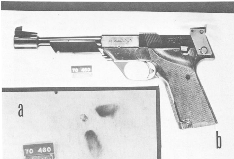
FIG. 2—(a) powder pattern on shirt; (b) weapon equipped with muzzle brake.
